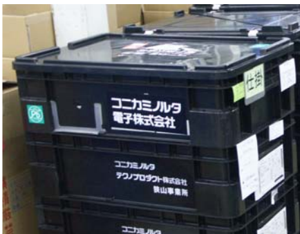
Returnable container that protects contents from static electricity
