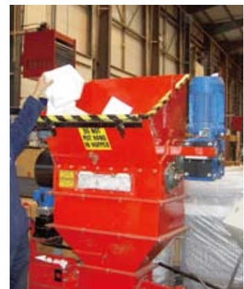
Foamed polystyrene pulverization machine
