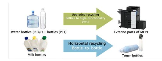
Konica Minolta also recycles milk containers made from polyethylene and turns them into toner bottles for MFPs. It has developed washing technology that removes the smell of milk and minute cells that would degrade the quality, and has established a mass production system in Mexico and Malaysia. The Company has succeeded in raising the percentage of PCR in the raw material used for toner containers to 40% and has attained 100% for some products.
